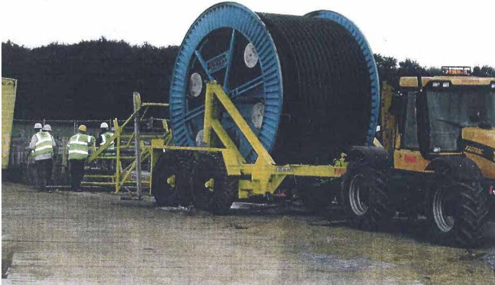
Figure 38 – Cable drum carrying trailer
